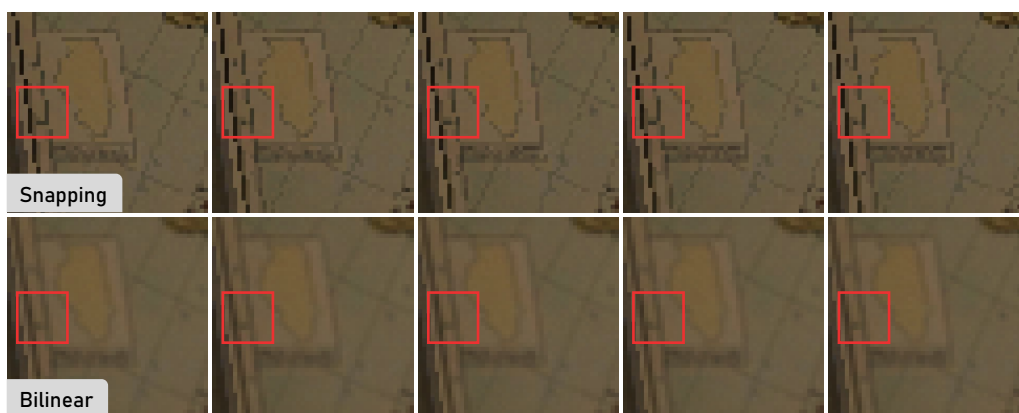
Figure 6.5: Comparison of the temporal stability of bilinear interpolation and nearest-neighbor interpolation with snapping. From left to right, the camera rotates one pixel to the right over five frames. Nearest neighbor interpolation causes visible changes in some texture details from one frame to another. Like in figure 6.4, the implicit anti-aliasing of the path tracer has been disabled here.
