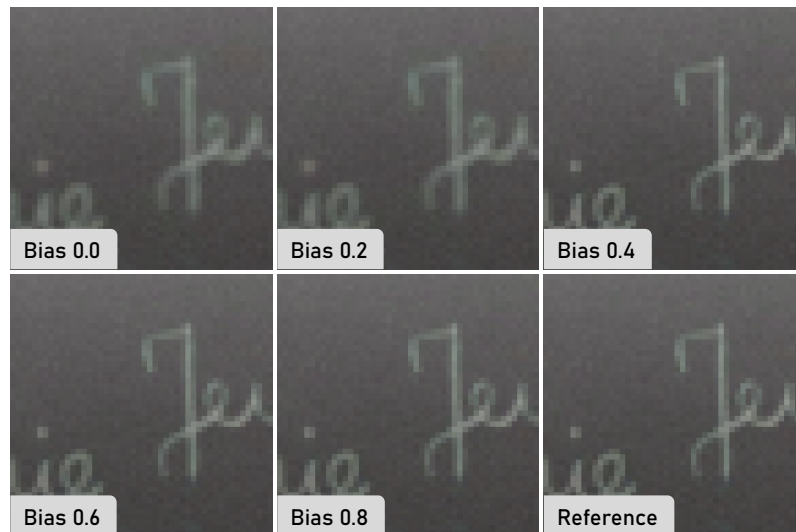
Figure 6.3: Applying a bias to the mipmap level of the virtual textures of the cache reduces the blur caused by bilinear interpolation.
